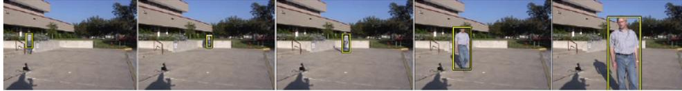
Figure 2.13: Mean shift tracking, proposed in (Collins, 2003).
